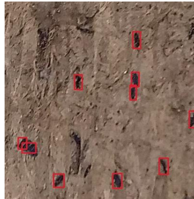
Figure 9. Example of the counting system output. Each red rectangle highlights a mosquito egg detected by the counting system.
