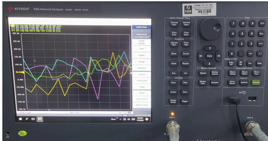
Figure 2 - Two-port VNA, model E5063A used for measurements.
