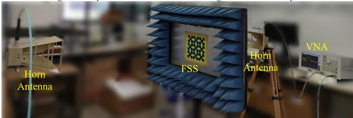
Figure 30 - Experimental measurement of FSS 1 using a vector network analyzer
