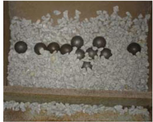
(b) Agregados com as esferas abrasivas
