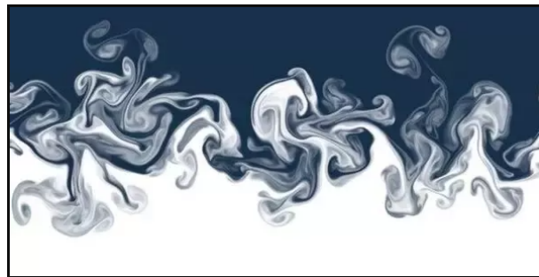
Figure 38 – . As the difference in density leads to instability, the heavier fluid interpenetrates the lighter one, as if the former was pushed by the later in a battle for occupying spaces.
