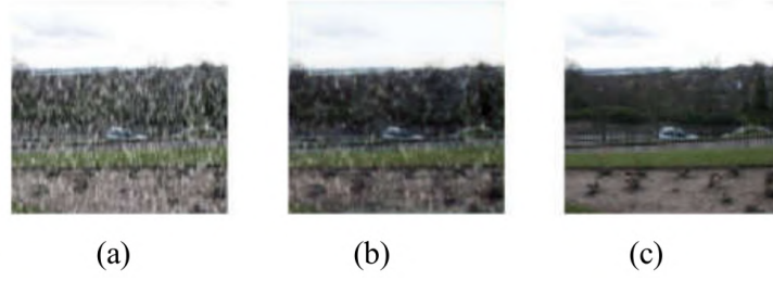
Figure 5 – a) Rain-Degraded Image b) U-Net c) Proposed U-Net based GAN method.
