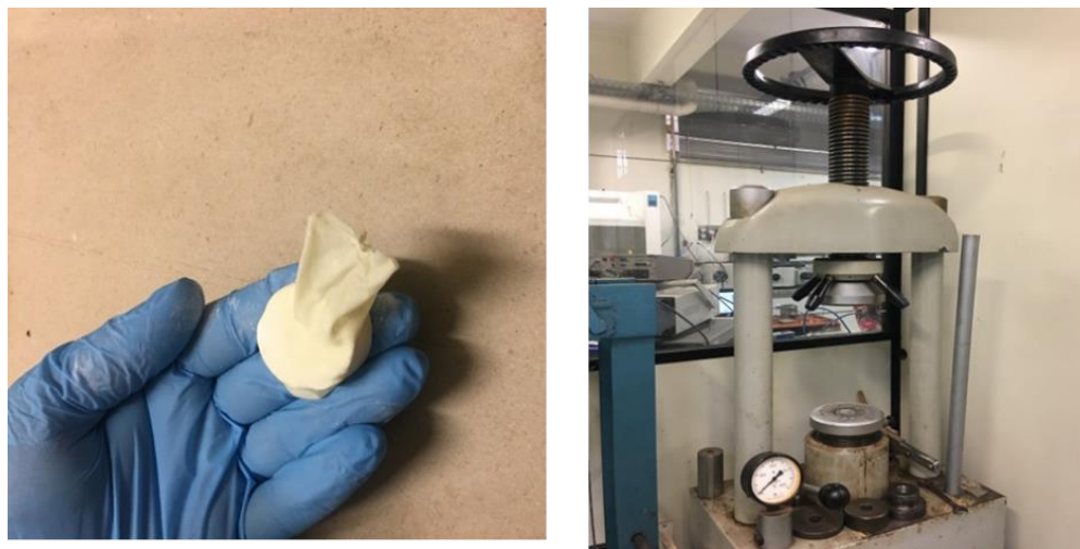
Figure 8: Hydrostatic pressure for reducing the spacing in pellet sintering process
