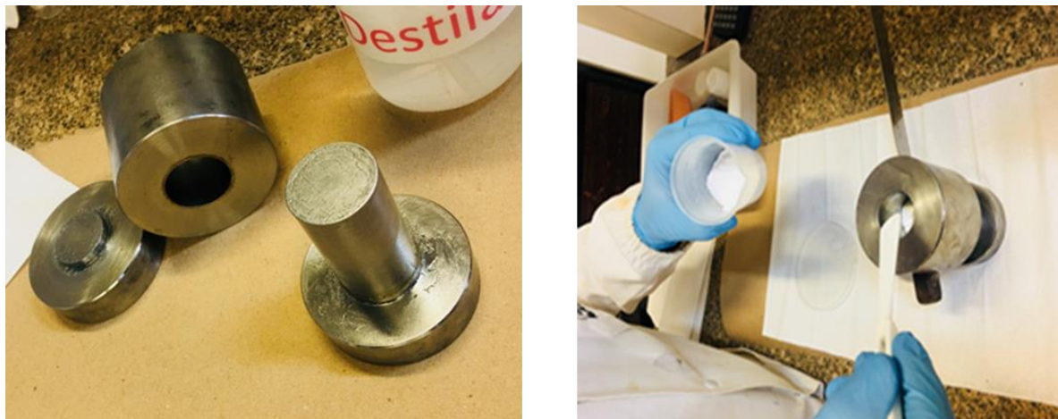
Figure 6 - Space holder to form the pellet and pouring the powder with certain shape
