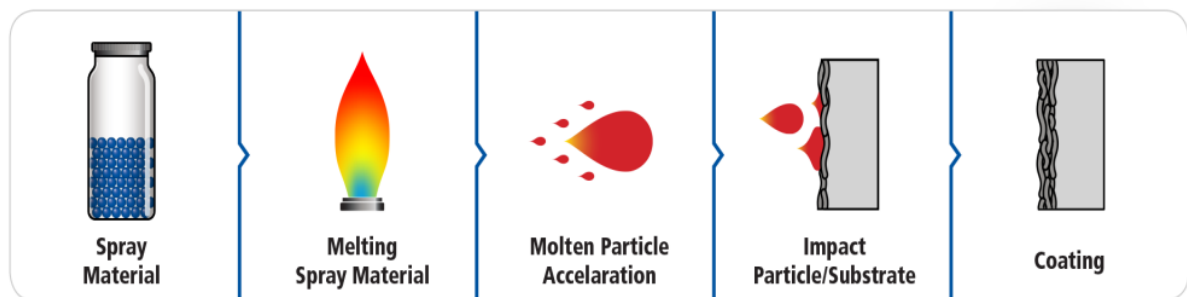
Figure 1 - Schamatic process of Thermal spray coating on the substrtae surface to adhere the particles
