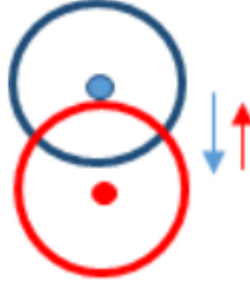
Figure 15: One possible scheme of non-composite vortex. The red vortex is in the first band and the red arrow indicating the direction to increase \Psi_1 . The blue vortex is in the second band and the blue arrow indicating the direction to increase \Psi_2 . Then r is calculated in a direction that \Psi_1 increase and \Psi_2 decrease, so r < 0 .
