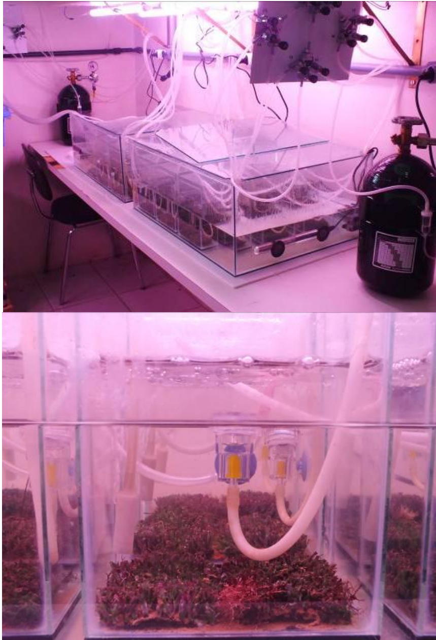
Fig. 4 a) Microcosm system illustrating aquariums with ASUs in water bath, and b) detail of ASUs and CO 2 diffuser
