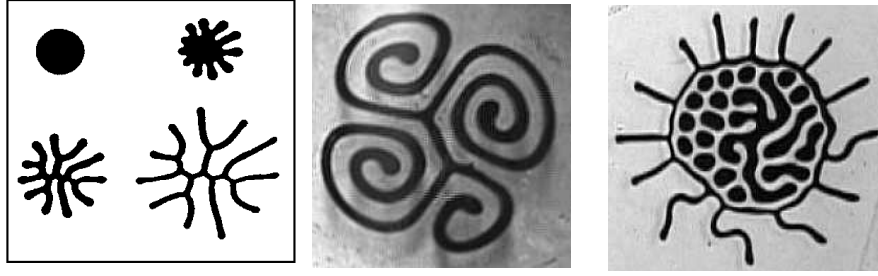
Figure 1.2: Ferrofluid viscous fingering patterns produced by different magnetic field configurations. The left panel [19] depicts the labyrinthine instability formed when a uniform magnetic field is applied perpendicularly to the plates. The mid and right panels [20] show spiral and protozoan-like shapes that arise when a rotating magnetic field is added to the perpendicular field.
