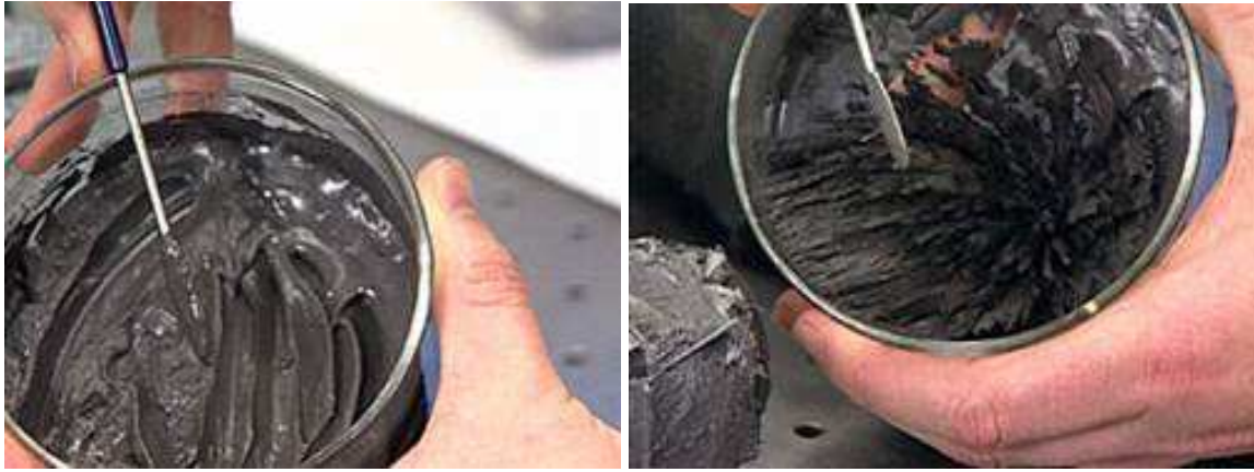
Figure 1.3: Magnetorheological fluid sample at the absence of an applied magnetic field (left) and at the presence of a magnet (right).
