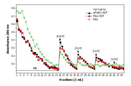
**Fig.2:** Affinity chromatography of human plasma protein using magnetic particle washed with phosphate buffer (PB) and increasing NaCl concentrations (0.25; 0.5; 1.0 M and 2.0 M).
