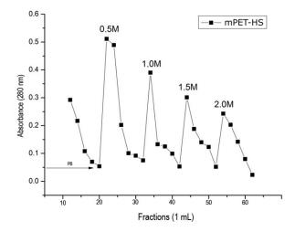
**Figure 2**: Affinity chromatography of human plasma proteins using ferromagnetic PET with heparan sulfate immobilized: mPET-HS was incubated with human plasma and washed with phosphate buffer ph 7.2, to balance the absorbance  $(280 \text{ nm}) - 20^{\text{th}}$  fraction: the particles were then washed with buffer containing increasing concentrations of NaCl (0.5M; 1.0M; 1.5M and 2.0M).
