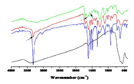
**Figure 1:** Infrared spectra of derivatives. In ascending order: magnetite; PET-hydrazide; mPET and mPET-HEP. 1: Band of NH<sub>2</sub> group of the hydrazide; 2: Band of amide I; 3: Band of amide II.
