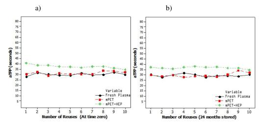
**Figura 4**: Activated partial thromboplastin time (aPTT) of fresh plasma performed by adding small aliquot of the eluate (1.0 M) of magnetic derivatives: a) Immediately synthesized (time zero) and b) 2 years stored at 4°C.
