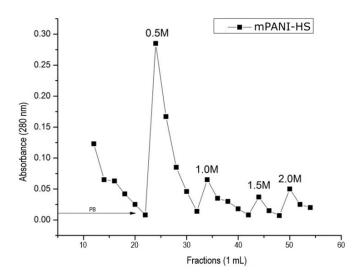
**Figure 1**: Affinity chromatography of human plasma proteins using magnetite coated with polyaniline and heparan immobilized: mPANI-HS was incubated with human plasma and washed with phosphate buffer ph 7.2, to balance the absorbance (280 nm) – 20<sup>th</sup> fraction: the particles were then washed with buffer containing increasing concentrations of NaCl (0.5M; 1.0M; 1.5M and 2.0M).
