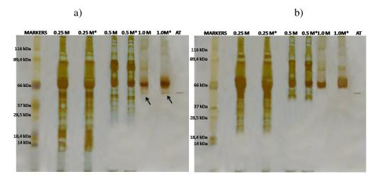
**Figure 2**: Electrophoresis of protein fractions of plasma obtained with the use of magnetic particles. Elutions were carried out using increasing NaCl concentrations (0.25; 0.5 and 1.0 M) in the magnetic derivatives: a) mPET-HEP and b) mPET (control). AT: Standard Antithrombin. \*Elutions performed in supports stored for 24 months. Arrows: Antithrombin (58 kDa).
