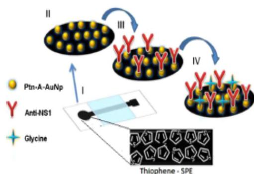
Fig. 1. Schematic illustration of the stepwise preparation of the NS1 immunosensor (I) bare thiophene-SPE; (II) AuNP-Ptn-A/thiophene-SPE; (III) anti-NS1/AuNP-Ptn-A/thiophene-SPE; and (IV) glycine/anti-NS1/AuNP-Ptn-A/thiophene-SPE.
