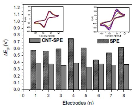
Fig. 2.  $\Delta E_p$  of the eight SPEs with and without  $\text{NH}_2\text{-CNT}$ . Inset: CVs of the electrodes with and without  $\text{NH}_2\text{-CNT}$  in presence of the  $\text{K}_3[\text{Fe}(\text{CN})_6]/\text{K}_4[\text{Fe}(\text{CN})_6]$  ( $5 \text{ mmol L}^{-1}$ ) prepared in PBS ( $10 \text{ mmol L}^{-1}$ , pH 7.4) at  $50 \text{ mV s}^{-1}$  scan rate.
