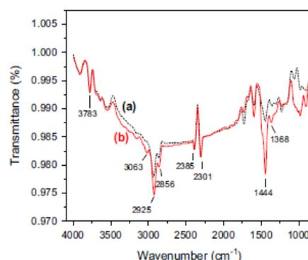
Fig. 3. ATR FT-IR spectra of the SPE (a) without  $\text{NH}_2\text{-CNT}$  and (b) with  $\text{NH}_2\text{-CNT}$ .
