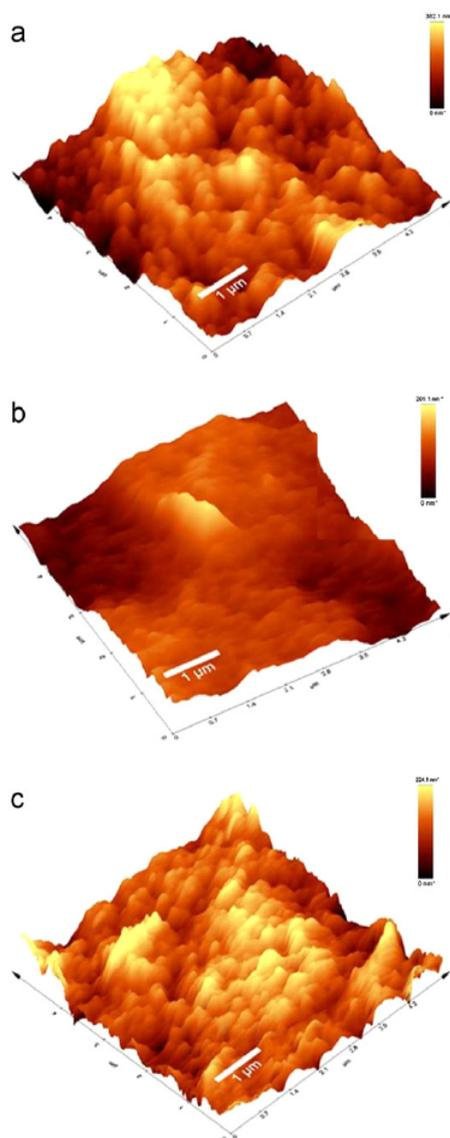
Fig. 3. AFM images: (a) bare CNT-SPE; (b) CNT-SPE modified by EDA and (c) CNT-SPE with immobilized anti-NS1.
