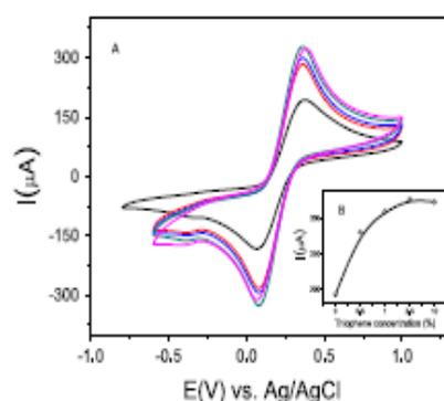
Fig. 4. Effect of the concentration of the thiophene monomer in the presence of  $5\text{ mmol L}^{-1}$  of  $\text{K}_3\text{Fe}(\text{CN})_6/\text{K}_4\text{Fe}(\text{CN})_6$  at a scanning rate of  $50\text{ mV s}^{-1}$ .
