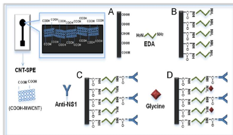
Fig. 2. Schematic illustration of the stepwise preparation of the immunosensor: (a) bare CNT-SPE, (b) EDA film formation, (c) anti-NS1 immobilization, and (d) blocking with glycine.
