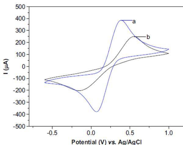
Fig. 1. Cyclic voltammograms profile of the carbon ink-printed electrode with CNT (a) and without CNT (b). Scans performed in 5 mmol L<sup>-1</sup> K<sub>3</sub>Fe(CN)<sub>6</sub>/K<sub>4</sub>Fe(CN)<sub>6</sub>, at 0.1 V s<sup>-1</sup> scan rate.
