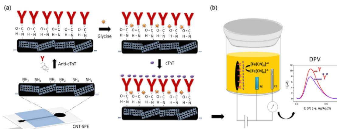
Fig. 1. Schematic representation of the (a) immunosensor fabrication and (b) electrochemical principle of detection.
