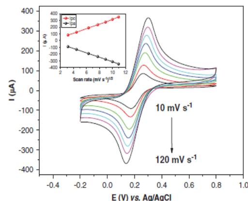
**Figure 2.** Voltammetric profile of the PAH/COOH-MWCNT/GCE in 5 mmol  $L^{-1}$   $K_3Fe(CN)_6/K_4Fe(CN)_6$  under different scan rates (10, 20, 40, 60, 80, 100 and 120  $mV s^{-1}$ ). Inset: Current at the anodic and cathodic peaks vs. square root of the scan rate.
