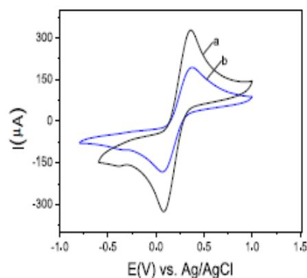
Fig. 2. (a) Cyclic voltammogram profiles of the carbon ink-printed electrode, with thiophene; and (b) without thiophene. The scans were performed in  $5\ \text{mmol L}^{-1}\ \text{K}_3\text{Fe}(\text{CN})_6/\text{K}_4\text{Fe}(\text{CN})_6$ , at a scanning rate of  $50\ \text{mV s}^{-1}$ .
