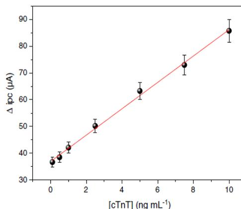
Fig. 9. Calibration curve of the immunosensor. The amperometry measurement was carried out in the  $\text{H}_2\text{O}_2$   $5 \text{ mmol L}^{-1}$  diluted in PBS  $10 \text{ mmol L}^{-1}$ , pH 7.0.
