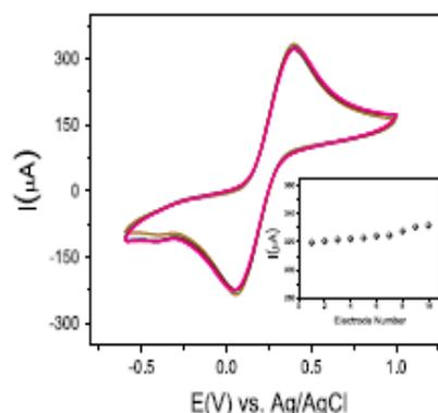
Fig. 6. Study of the reproducibility and stability of printed electrodes modified with thiophene. Ten screen-printed electrodes were tested in the presence of  $5\text{ mmol L}^{-1}$  of  $\text{K}_3\text{Fe}(\text{CN})_6/\text{K}_4\text{Fe}(\text{CN})_6$  at a scanning rate of  $50\text{ mV s}^{-1}$ .
