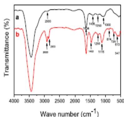
Fig. 5. ATR-FTIR spectra of the SPE—(a) without thiophene; and (b) with thiophene.
