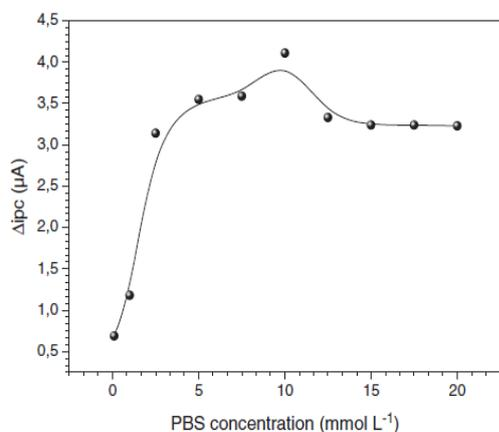
Fig. 7. Effect of PBS concentration on the immunosensor response. The amperometry measurement was carried out in the  $\text{H}_2\text{O}_2$   $5 \text{ mmol L}^{-1}$  (pH 7.0).
