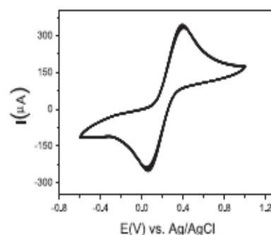
Fig. 3. Cyclic voltammograms of the thiophene-SPE from twenty replicate cycles performed in presence of  $5\ \text{mmol L}^{-1}$  of  $\text{K}_3\text{Fe}(\text{CN})_6/\text{K}_4\text{Fe}(\text{CN})_6$  prepared in a  $0.1\ \text{mol L}^{-1}$  KCl solution, at a scanning rate of  $50\ \text{mV s}^{-1}$ .
