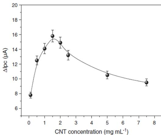
Fig. 4. Influence of the CNT concentration on the cathodic peak current. CVs were conducted in a solution of 4  $\text{mmol L}^{-1}$   $\text{K}_3\text{Fe}(\text{CN})_6$ .
