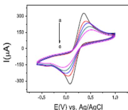
Fig. 8. Cyclic voltammograms of the immunosensor in each step of immobilization: (a) bare thiophene-SPE; (b) AuNP-Ptn-A/thiophene-SPE; (c) anti-NS1/AuNP-Ptn-A/thiophene-SPE; (d) glycine/anti-NS1/AuNP-Ptn-A/thiophene-SPE and (e) NS1/glycine/anti-NS1/AuNP-Ptn-A/thiophene-SPE. Scans were performed in  $5 \text{ mmol L}^{-1}$  of  $\text{K}_3\text{Fe}(\text{CN})_6/\text{K}_4\text{Fe}(\text{CN})_6$  at a scanning rate of  $0.1 \text{ V s}^{-1}$ .
