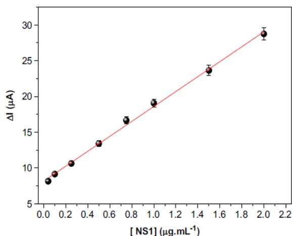
Fig. 5. Calibration curve of the immunosensor for NS1 protein of dengue virus.
