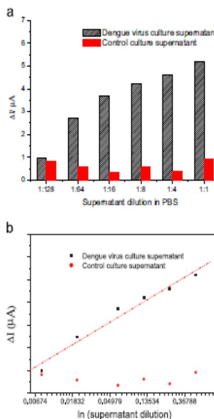
Fig. 10. (a) Analytical responses of thiophene-SPEs to the NS1 native protein f from dengue virus and control (CD4 cells) culture supernatant at serial dilutions. (b) Linear fit obtained by natural logarithm of supernatants dilutions. The amperometric responses obtained by DDP in  $5 \text{ mmol L}^{-1}$  of  $\text{K}_3\text{Fe}(\text{CN})_6/\text{K}_4\text{Fe}(\text{CN})_6$ .
