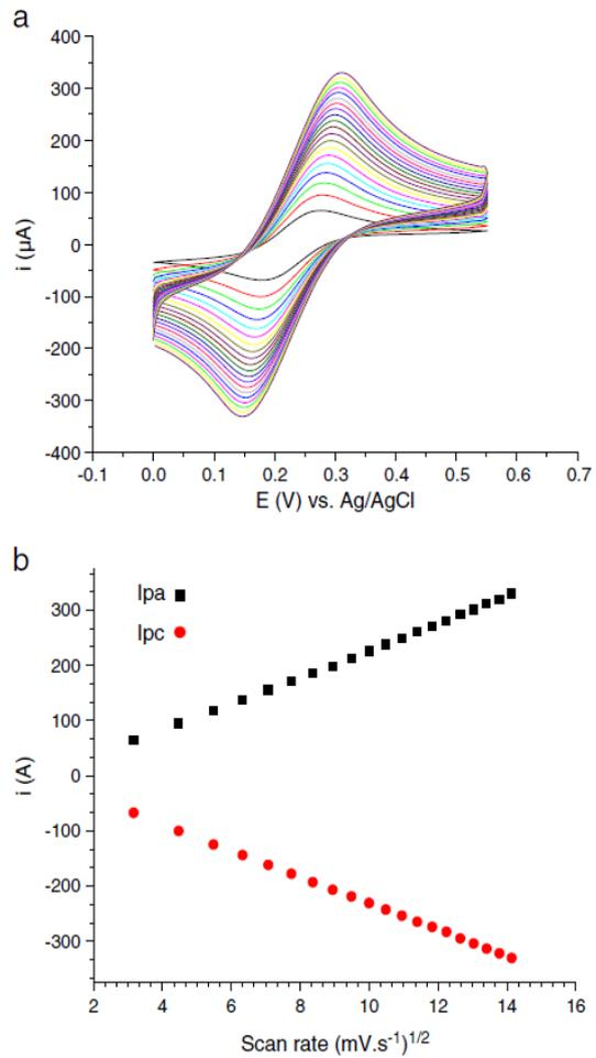
Fig. 5. (a) Cyclic voltammograms of the immunosensor in the 4  $\text{mmol L}^{-1}$   $\text{K}_3\text{Fe}(\text{CN})_6$  at scan rate (from inner to outer): 10, 20, 30, 40, 50, 60, 70, 80, 90, 100, 110, 120, 130, 140, 150, 160, 170, 180, 190, 200  $\text{mV s}^{-1}$  (b) Plots of currents peak as a function of square root of scan rate.
