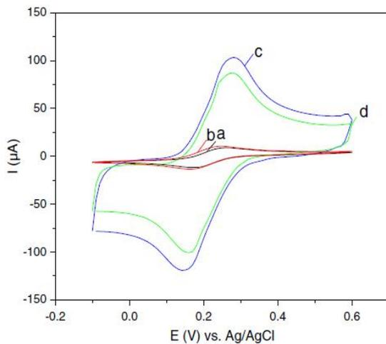
Fig. 2. Cyclic voltammograms of the immunosensor in each step of immobilization: (a) bare Au, (b) PEI/Au, (c) CNT/PEI/Au, (d) anti-cTnT/CNT/PEI/Au, in the presence of  $4 \text{ mmol L}^{-1} K_3Fe(CN)_6$  under scan rate of  $100 \text{ mV s}^{-1}$ .
