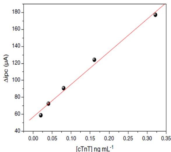
Fig. 10. Linear response of immunosensor to the serum samples in different concentrations of cTnT measured by ECLIA methods.
