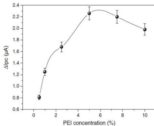
Fig. 3. Effect of the PEI concentration on the immunosensor response. Measurements were conducted by CV in a solution of  $H_2O_2$   $5 \text{ mmol L}^{-1}$  diluted in PBS  $10 \text{ mmol L}^{-1}$ , pH 7.0.
