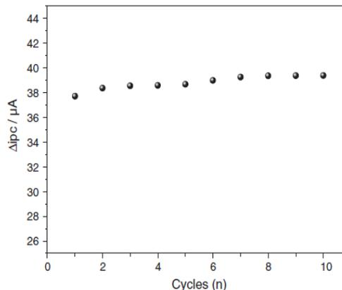
Fig. 8. Repeatability of the immunosensor in ten replicate measurements.
