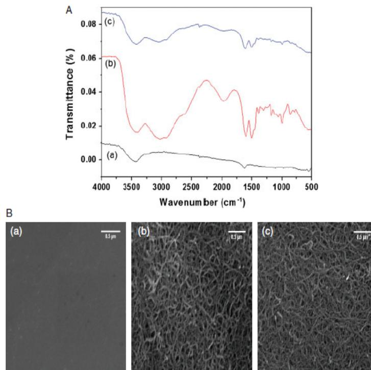
**Figure 3.** (A) FTIR spectra in transmission mode (a) COOH-MWCNT, (b) PAH, (c) PAH/COOH-MWCNT and (B) SEM images of (a) bare GCE, (b) GCE modified with COOH-MWCNT and (c) GCE modified with COOH-MWCNT and PAH.
