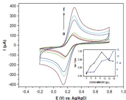
**Figure 1.** Cyclic voltammograms of the electrode modified with different COOH-MWCNT droplet size: (a) bare GCE; (b) 2.5  $\mu L$ ; (c) 5  $\mu L$ ; (d) 10  $\mu L$ ; (e) 15  $\mu L$ ; and (f) 17.5  $\mu L$ , in the presence of 5 mmol  $L^{-1}$   $K_3Fe(CN)_6/K_4Fe(CN)_6$  at a scan rate of 100  $mV s^{-1}$ . Inset:  $I_{pc}/I_{pa}$  (solid line) and area (dashed line) depending on the COOH-MWCNT droplet size.
