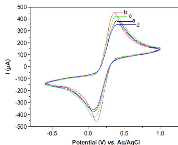
Fig. 4. Cyclic voltammograms of the immunosensor in each step of immobilization: (a) bare CNT-SPE; (b) EDA/CNT-SPE; (c) anti-NS1/EDA/CNT-SPE and (d) glycine/anti-NS1/EDA/CNT-SPE. Scans performed in  $5 \text{ mmol L}^{-1} \text{ K}_3\text{Fe}(\text{CN})_6/\text{K}_4\text{Fe}(\text{CN})_6$  at  $0.1 \text{ V s}^{-1}$  scan rate.
