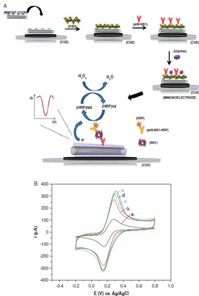
**Figure 4.** (A) Principle of the amperometric immunosensor showing the stepwise construction of immunoelectrode and principle of immunoassay. (B) Cyclic voltammograms at (a) bare GCE, (b) COOH-MWCNT/GCE, (c) PAH/COOH-MWCNT/GCE, (d) anti-NS1/PAH/COOH-MWCNT/GCE, (e) glycine/anti-NS1/PAH/COOH-MWCNT/GCE. The scans were performed in  $5 \text{ mmol L}^{-1} \text{ K}_3\text{Fe}(\text{CN})_6/\text{K}_4\text{Fe}(\text{CN})_6$ , at  $100 \text{ mV s}^{-1}$  scan rate.
