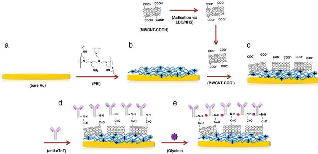
Fig. 1. Schematic diagram of the immunosensor in the successive steps. (a) Bare Au, (b) formation of the PEI film, (c) assembly of the COOH-CNT, (d) immobilization of anti-cTnT, (e) blocking with glycine.
