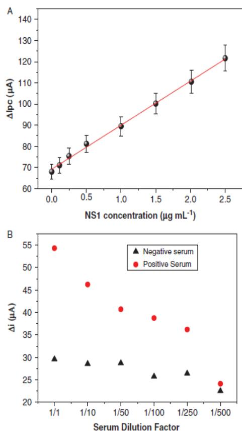
**Figure 5.** (A) Calibration curve of the immunosensor for NS1 antigen. (B) Response to the NS1 in negative and NS1 spiked serum samples at different PBS dilutions.
