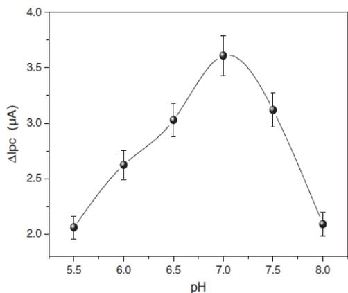
Fig. 6. pH effect on the immunosensor response. The amperometry measurement was carried out in  $\text{H}_2\text{O}_2$   $5 \text{ mmol L}^{-1}$ .
