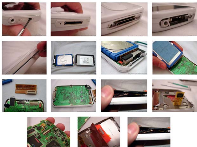
Figure 12. Steps show how to disassemble a MP4 player (Anythingbutipod, 2006).
