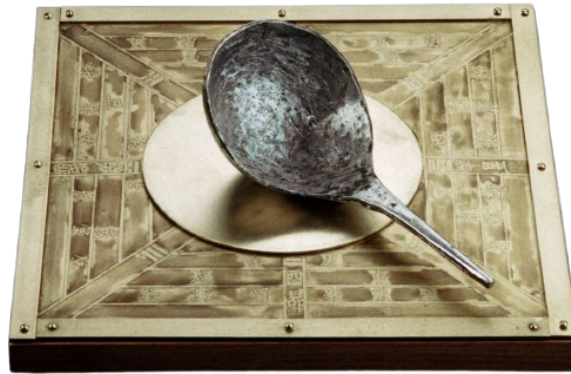
Figure 1 – Replica of the Chinese south-pointing spoon ( Si Nan or “south seeker”), an object thought to be a precursor to the magnetic compass approximately 2000 years ago during China’s Han dynasty and, in those days, associated with the divine.
