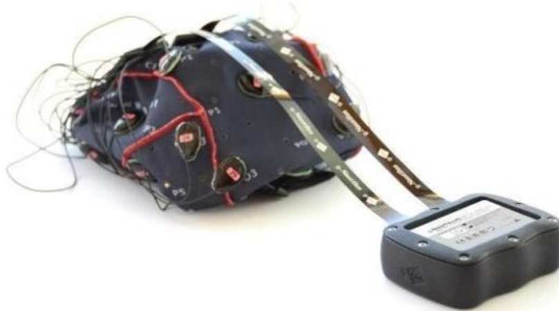
Figura 12. Nautilus Research , wearable EEG headset (32 canais).
