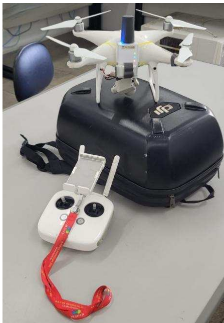
Figura 4 – DJI Phantom 4 Advanced com Kit PPK2
