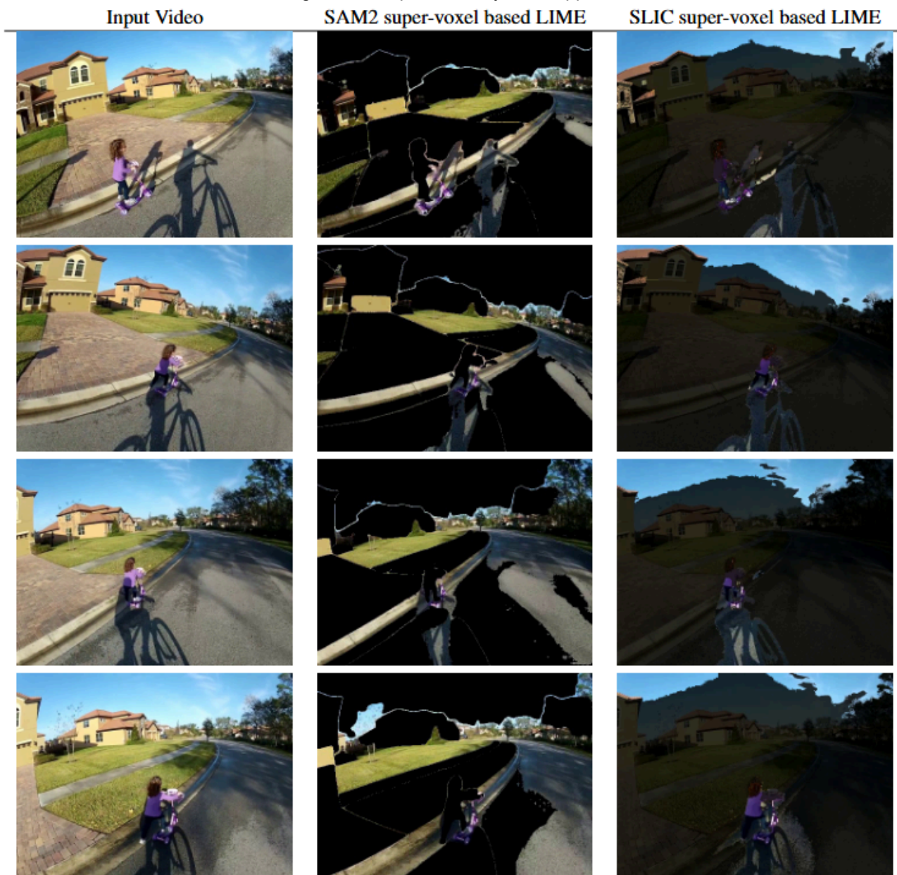
Figure 3 – The predicted action in this video is "riding scooter." In this comparison, neither method shows a clear advantage; results appear subjective. However, SAM2 generates well-defined boundaries around clusters, whereas the segmentation produced by SLIC appears more concentrated.
