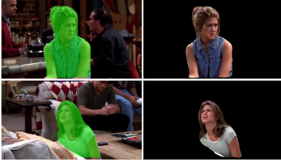
Figure 25 – The proposed approach to deal with the cluttered background problem. We regress a mask around the main performer to occlude the background information (left column) using Mask R-CNN (HE et al., 2017) and force the keypoints detection model to focus on the foreground information. If more than one mask is regressed on the image, we use the face crop region to select the correct mask. The output is the image with only the main performer’s body present (right column).
