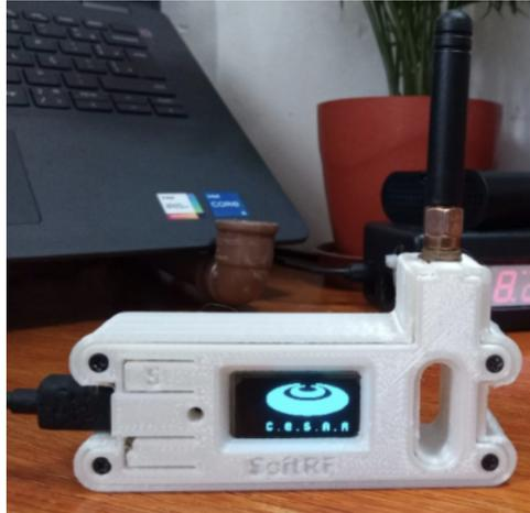
**Figura 4.7** End Device Esp32 LoRa Oled Heltec.
