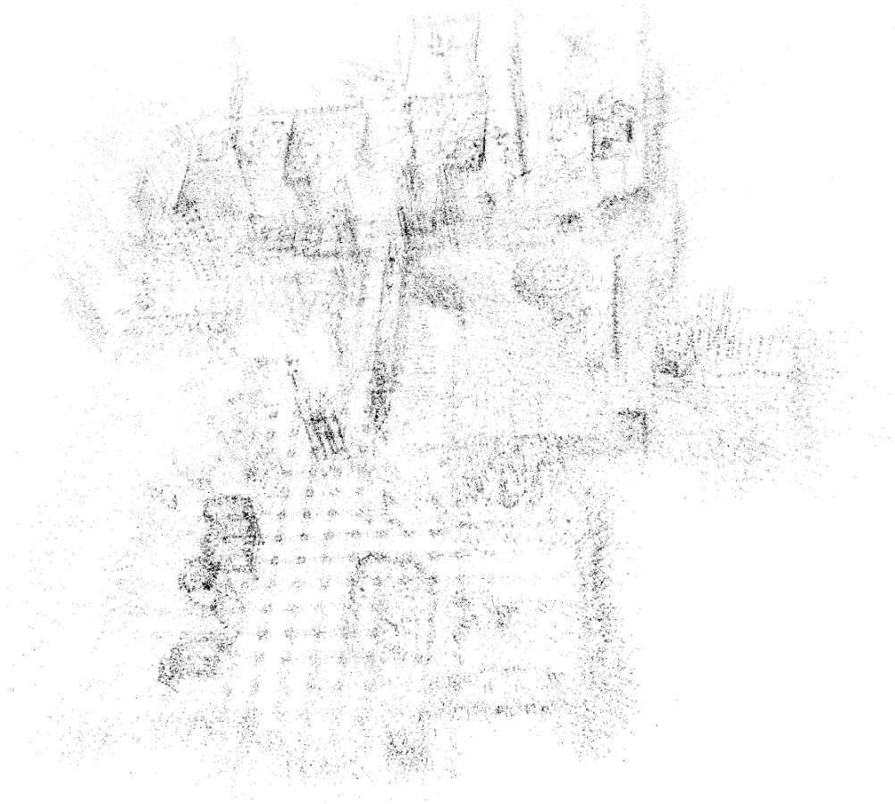
Figure 21 – A close-up view of the feature-based 3D metric map generated for path home_rz using ORB-SLAM2.
