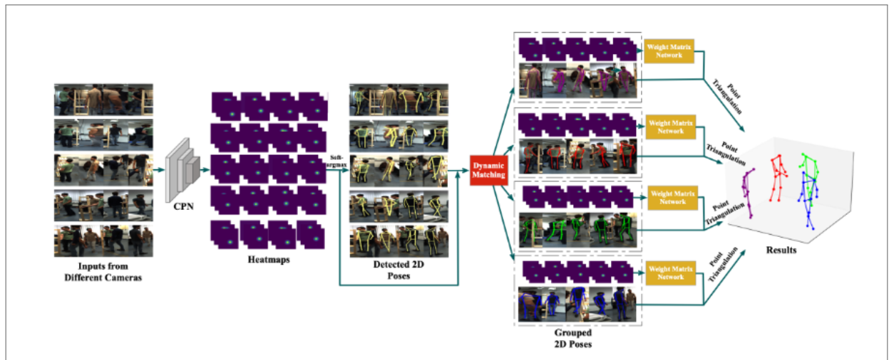
Figure 22 – The framework of (HUANG et al., 2020). The images are the input into to the 2d poses estimator (HUANG et al., 2020) to get the heatmaps. Next, they apply soft-argmax on heatmaps to get the corresponding 2d poses. Then, they feed both heatmaps and 2D estimated poses into matching module. They then sent the heatmaps into a network to get weight matrices. Finally, each cluster is sent to a weight-sharing 3d pose estimator to get the 3D pose.
