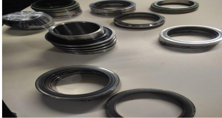
Figure 13: Internal components (gland seal, packing seal and wear rings)
