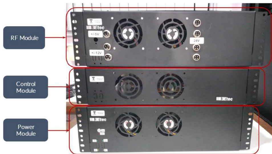
Figure 11 Encapsulation of intelligent antenna array control system devices.
