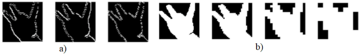
Figure 40 – a) 1st decomposition result for LH, HL and HH bands and (b) Approximation coefficients matrix image from (THALANGE; DIXIT, 2016).
