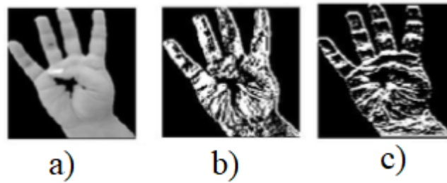
Figure 39 – a) Cropped gray image, b) and c) are the dx and dy results from (THALANGE; DIXIT, 2016).
