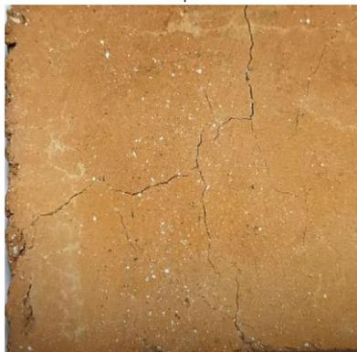
Figura 114 - Mistura 3 |Ataque  $\text{NH}_4\text{Cl}$ .
