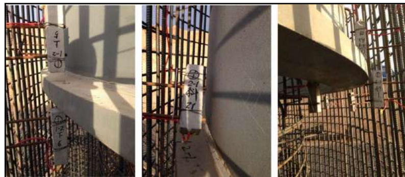
Figure 18 – Strain sensors installed around the flange of the embedded ring.
