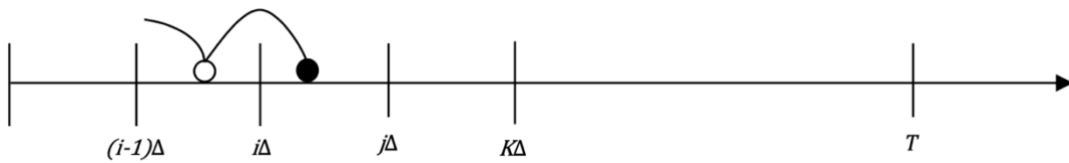
Figure 30 – Model 3, case 8. Symbol key: defect arrival ( \circ ); and failure ( \bullet ).
