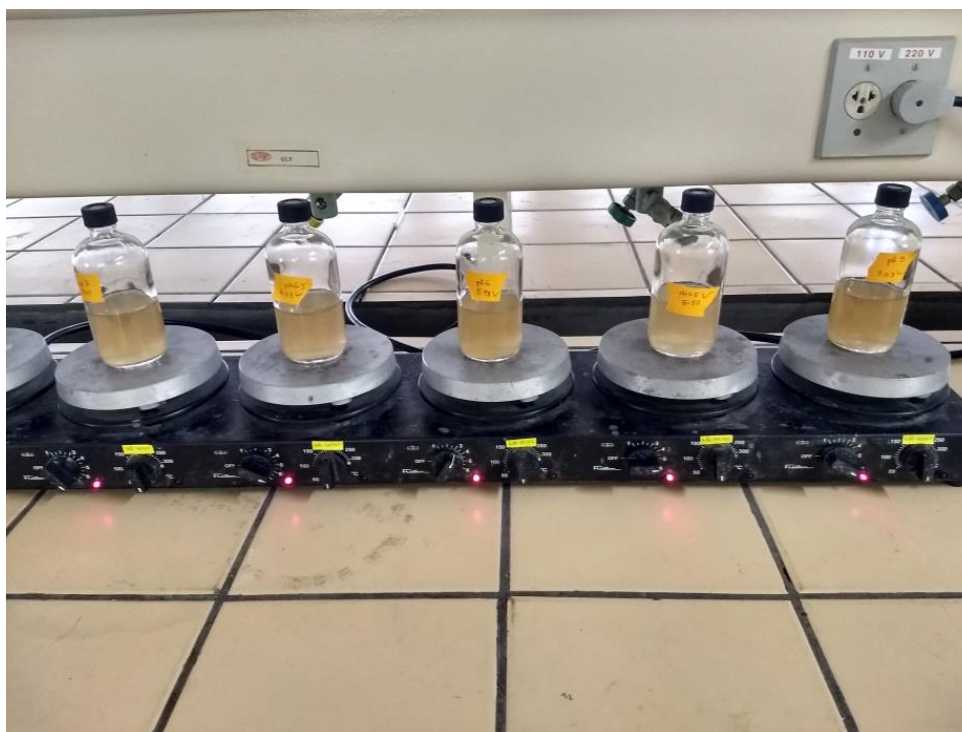
Figure 90C - Microcosms set for activity test of E-CS under different initial values of pH
