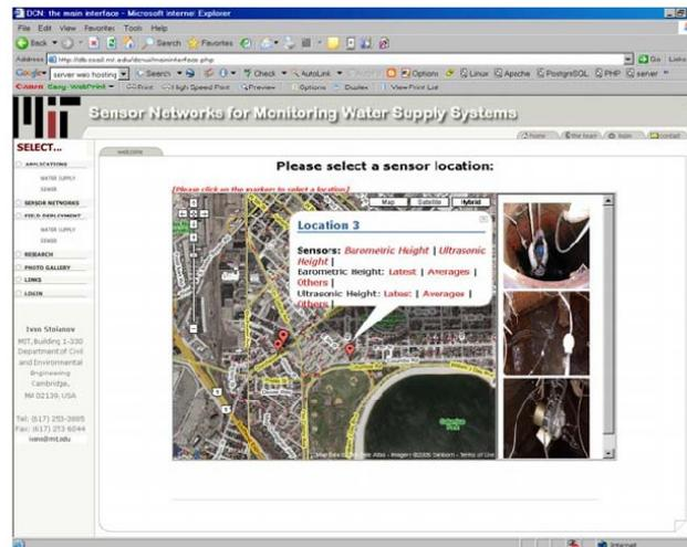
Figure 8: Web interface including Google MAP API for geospatial viewing of sensor data
