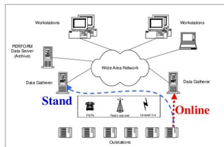
Figure 1: Schematic of a SCADA system
