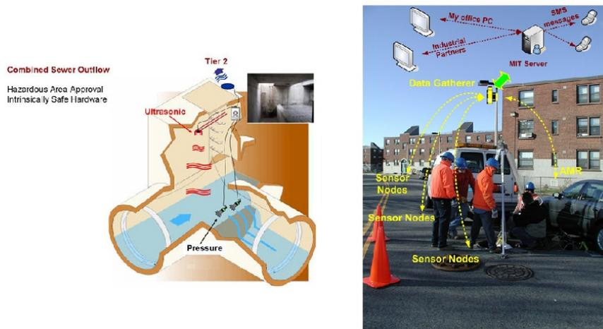
Figure 11: Figure: Schematic of Cluster 3, CSO monitoring
