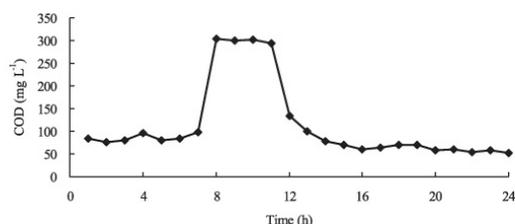
Fig. 7. COD concentrations in the outflow from the wastewater treatment plant on 30 August 2005.
