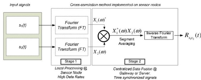
Figure 6: Procedure for calculating the cross-correlation function
