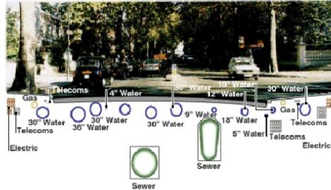
Figure 2: Underground infrastructure in urban environment. (Courtesy of Thames Water Ltd).
