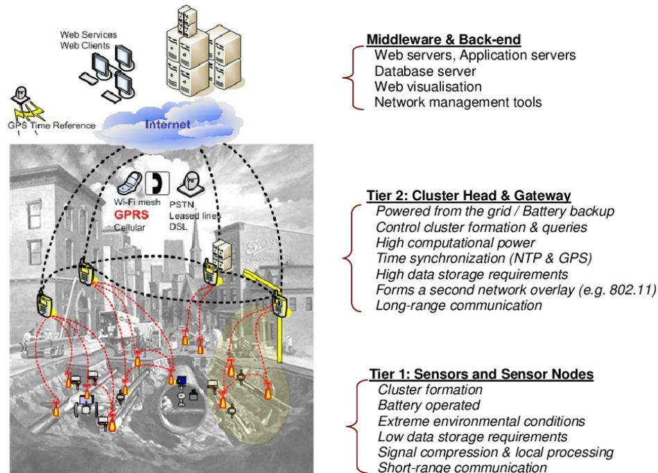
Figure 7: Schematic of the three tiers of the developed monitoring system
