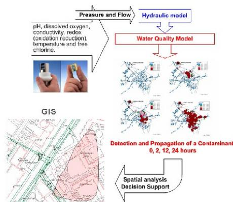
Figure 4: Simulation of the spread of a contaminant over time
