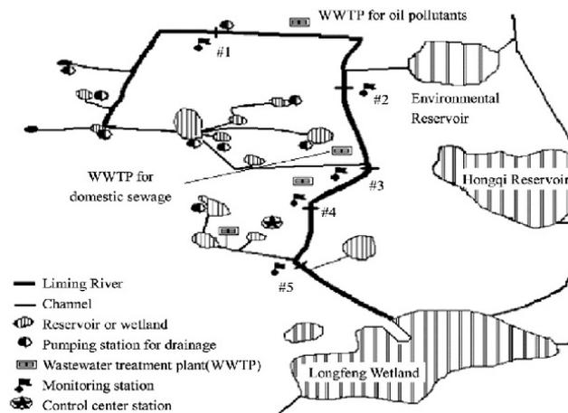
Fig. 1. Schematic diagram of the Liming River basin.
