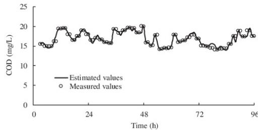
Fig. 4. Results of the training and learning stages for the ANN used to estimate COD (with pH in the range of 4.3–6.2).
