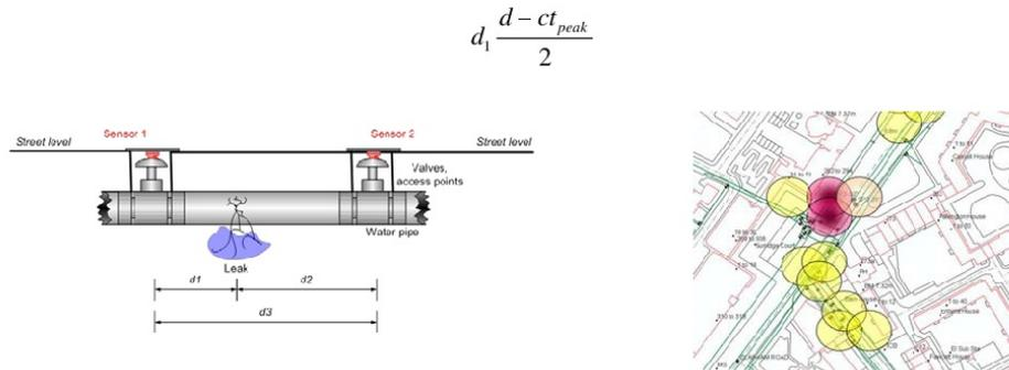
Figure 5: Acoustic leak detection (fixed point remote monitoring)
