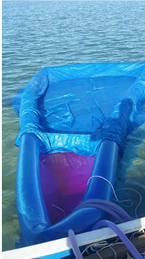
Figure 4 – Inflatable pool used during the experiment, filled with seawater mixed with rhodamine WT and NaOH.
