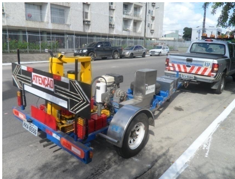
Figura 4 - Falling Weight Deflectometer (FWD)
