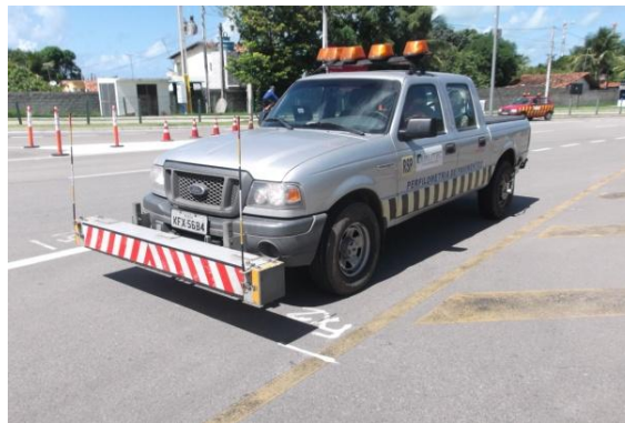
Figura 6 - Road Surface Profiler (RSP)
