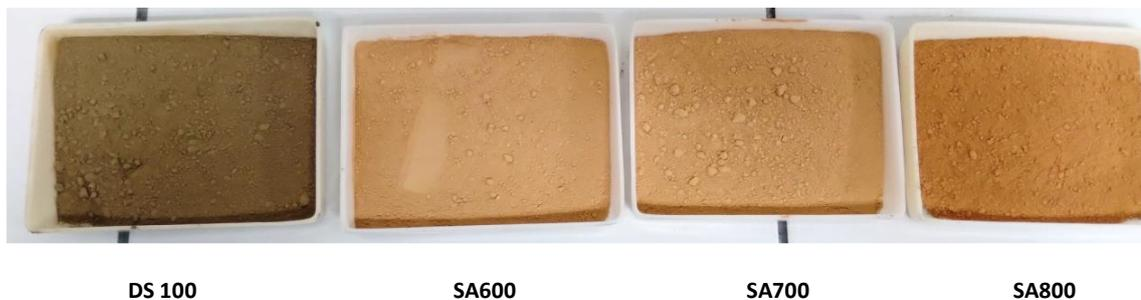
**Figure 1** – Appearance of dried (DS100) and calcined (SA600, SA700, and SA800) water treatment sludge after grinding.
