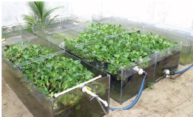
Figure 3. Experimental arrangement of free water surface flow constructed wetlands populated by *Eichhornia crassipes*.
