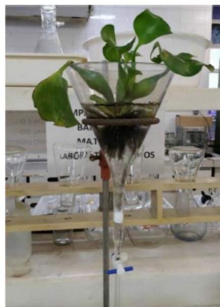
**Fig. 1** Experimental apparatus used for biosorption studies with  $80 \pm 5$  g of *E. crassipes* and 500 mL of synthetic oily effluent
