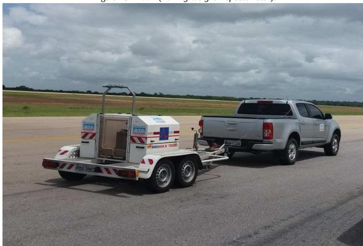
Figura 45 - FWD ( Falling Weight Deflectometer ).
