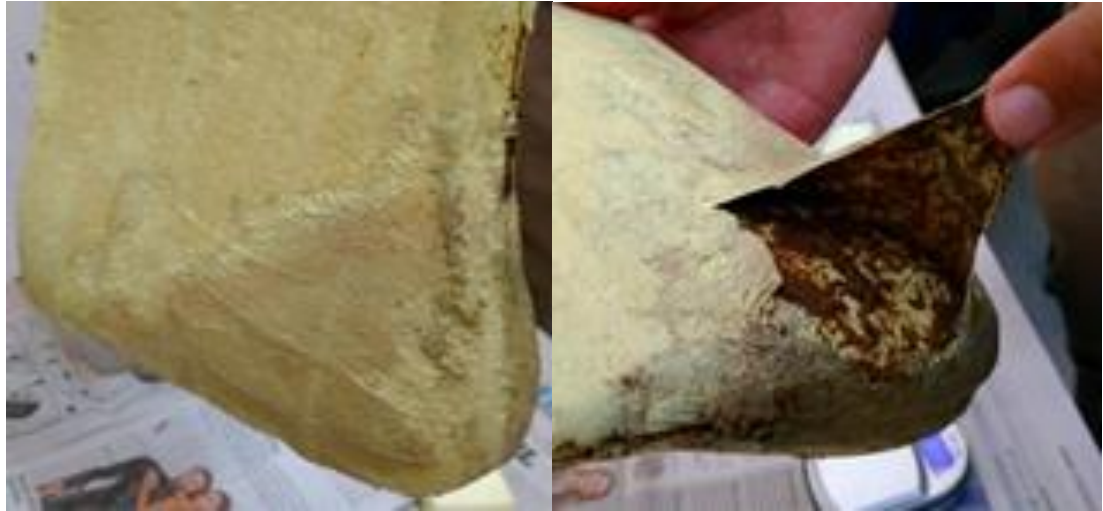
Figure 69 – Partial model after the water tightness test.
