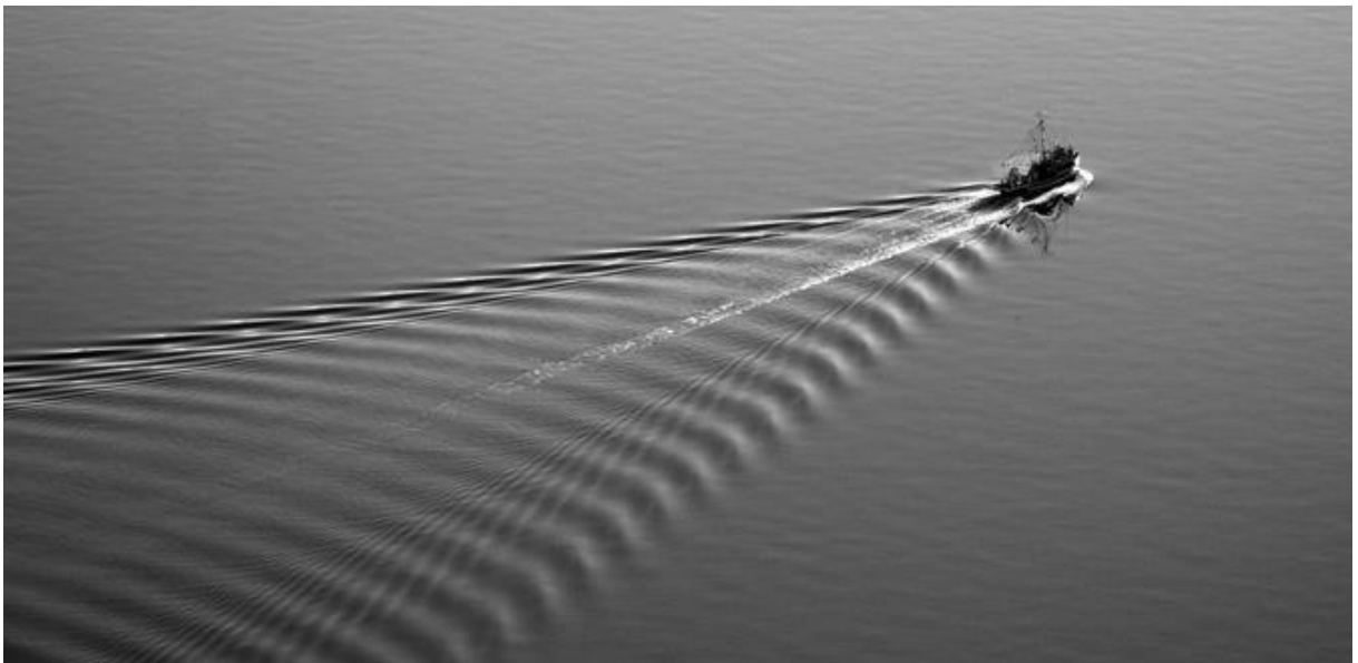
Figure 9 – Ship's wave pattern
