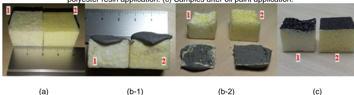
Figure 67 – Tests of two plastics against polyester resin and oil paint. “1” refers to “Plastic 1” and “2” to “Plastic 2”. (a) Samples with size: 20 mm × 20 mm × 15 mm before tests. (b-1), (b-2) Samples after polyester resin application. (c) Samples after oil paint application.
