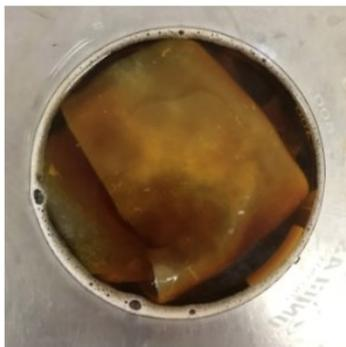
Figure 1: BC membrane being purified on NaOH.
