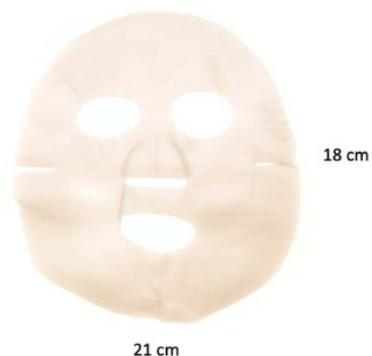
Figure 3 Prototype of the BioMask made out of BC with propolis extract
