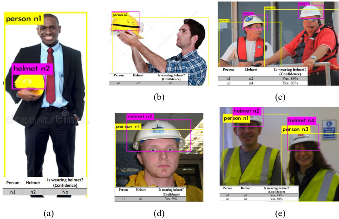
Figure 23 - PPE usage detection based on SVM.
