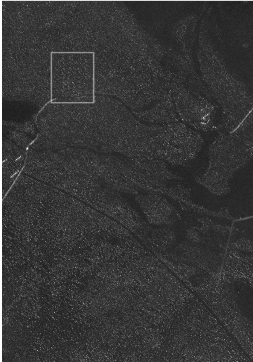
Figure 28 – Ground scene prediction image for Stack 1 based on the mean method. The areas highlighted by rectangles in the images indicate the regions where the targets were deployed during the measurement campaign.
