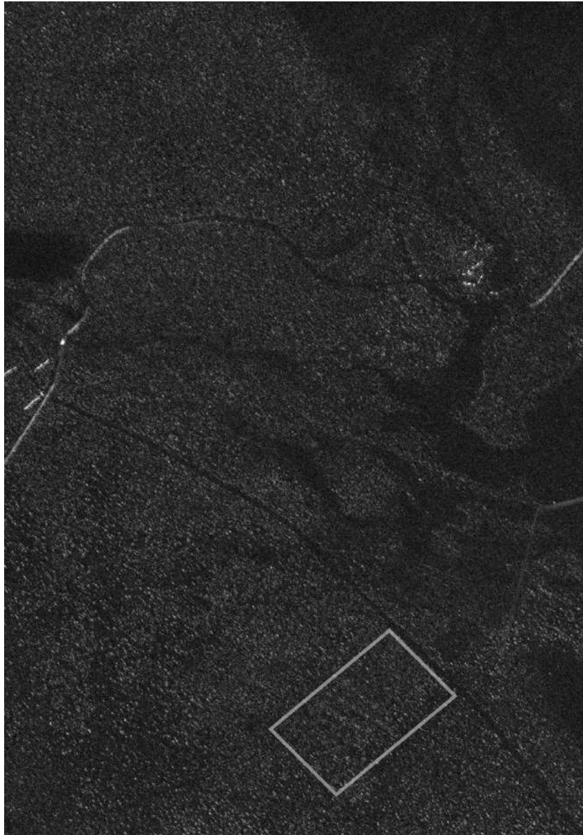
Figure 25 – Ground scene prediction image for Stack 1 based on the AR model. The areas highlighted by rectangles in the images indicate the regions where the targets were deployed during the measurement campaign.
