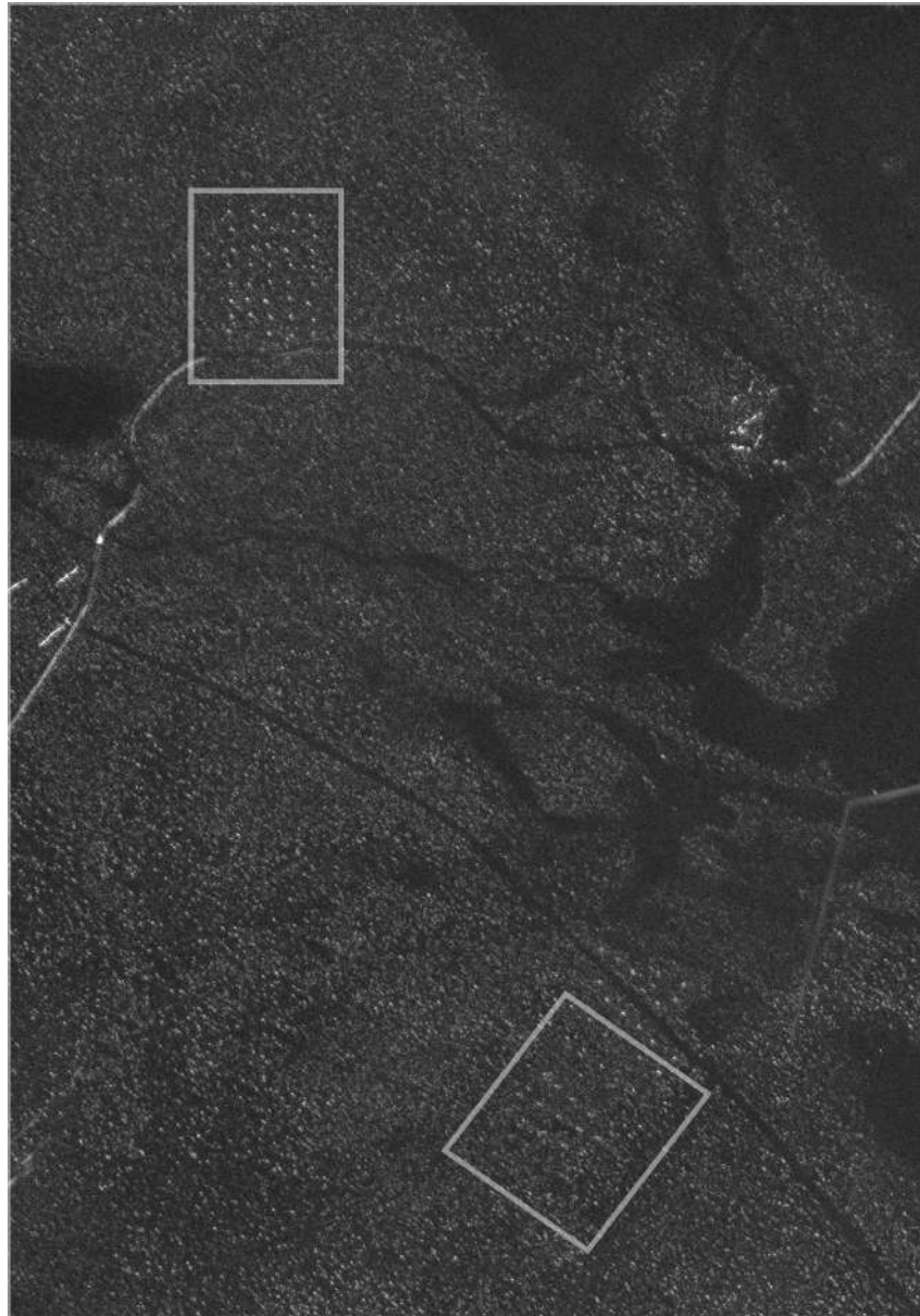
Figure 29 – Ground scene prediction image for Stack 1 based on the intensity mean method. The areas highlighted by rectangles in the images indicate the regions where the targets were deployed during the measurement campaign.
