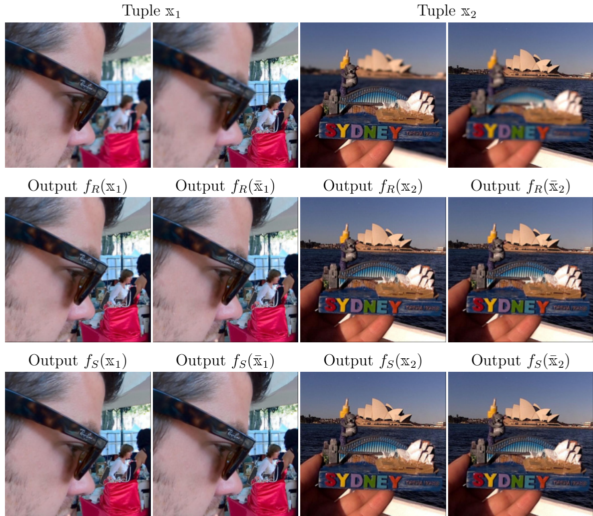
Figure 46 – Example of fusion results for tuples with normal and reversed order. In the first row are shown the frames within the tuples. In second and third row are shown the fusion results with the regression and segmentation networks respectively for both normal and reverse order evaluations.
