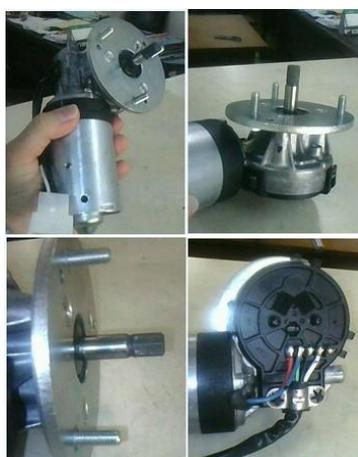
**Figura 39** – Motor DC BOSCH de 12 V/50W /35-50 rpm
