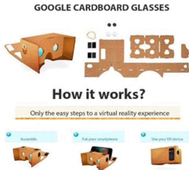
Figure 18 - Google cardboard Glasses, Low-cost adaptation for smartphones to function as devices of VR
