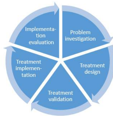
Figure 10 – The engineering design cycle (adapted from Wieringa (2010)).
