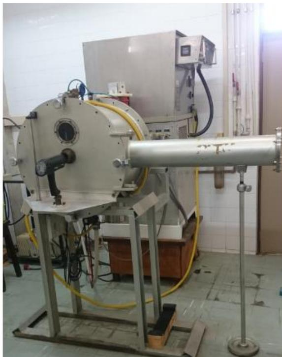
**Figura 20: Melt spinning**
