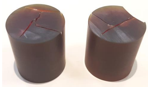
Figure 26: Cracked sample [3°C/min, 110°C, 2h].
