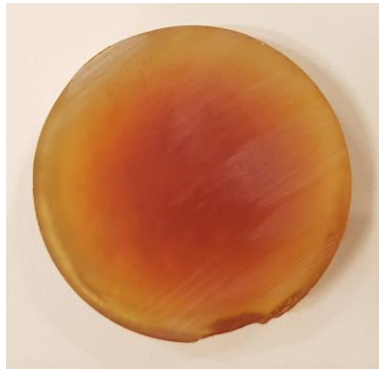
Figure 10: LY 556 epoxy cylinder of 32 mm diameter cured with an isotherm of 140°C: (a) bottom-cut surface and (b) full cylinder.
