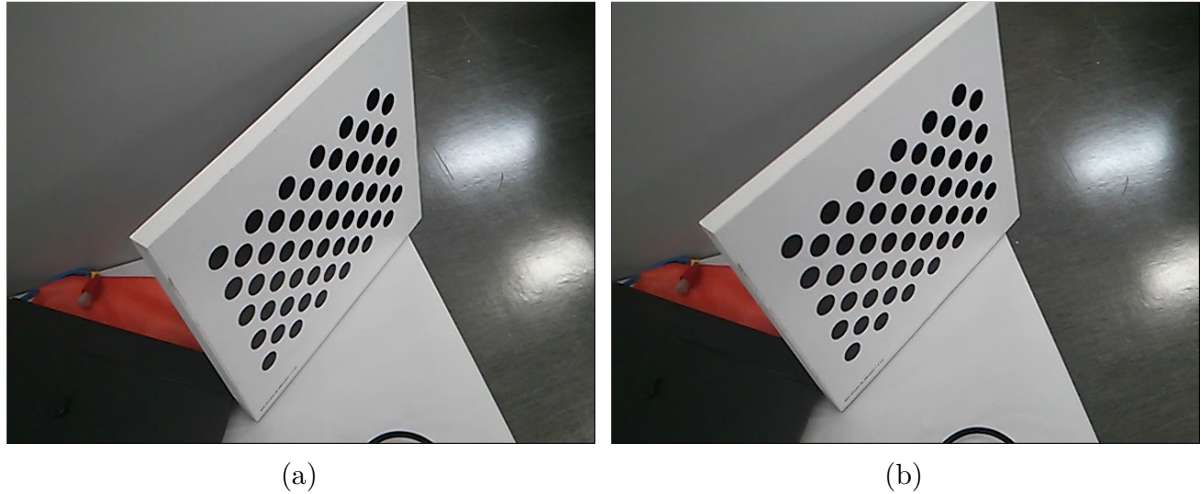
Figure 63 – The input image 0070 (the first of the obliquity set) is in (a); it has not been detected by the proposed detector because of its distortion. The next image of the set (the image 0088) is in (b); from this image proposed succeed.
