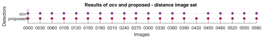
Figure 59 – Pattern detectors results for image set distance . The result of each detector is presented on a per-image basis; the presence of a circle indicates that the detector succeeded in that frame. Images are identified by four-digit names drawn from their original frame numbers in the video footage.
