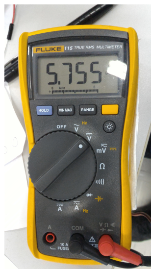
Figure 4.9: Voltage measured on the output of the voltage regulator with a 360\Omega resistor.
