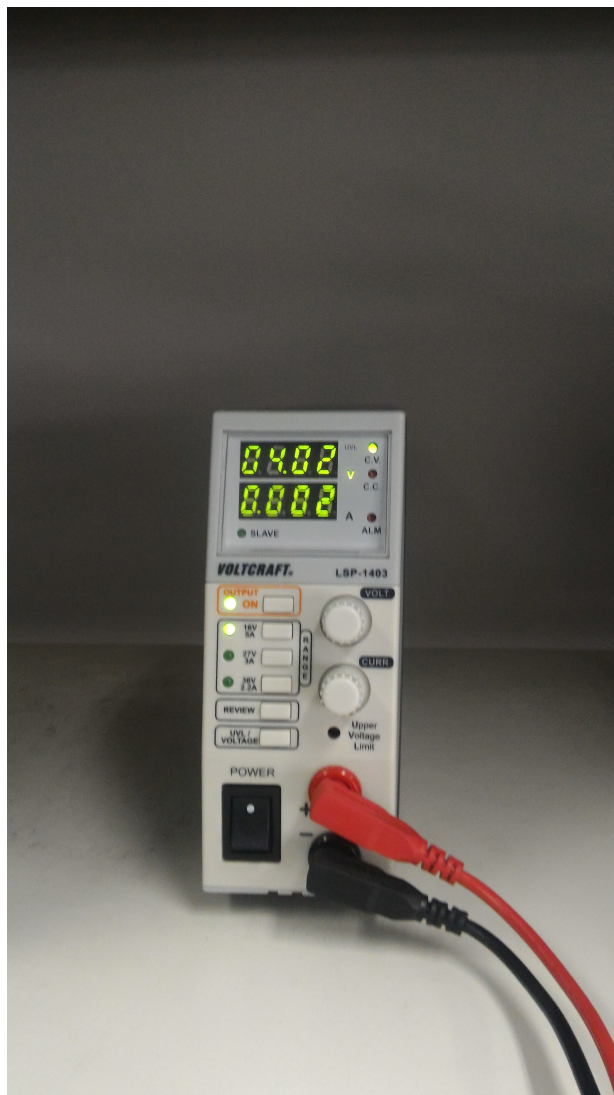
Figure 4.3: Picture of the voltage generator when a load is pulling 2mA@4V.
