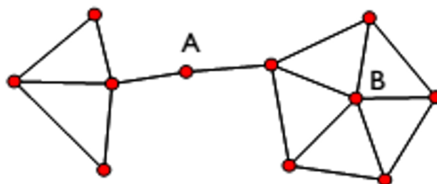
Figure A.6: Differences between high local centrality (node B) and high betweenness centrality (node A)
