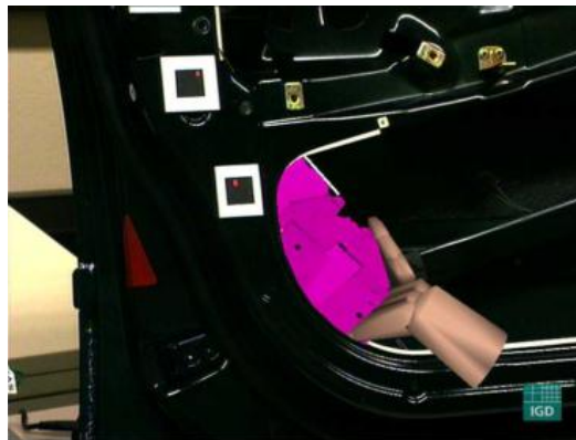
Fig. 34. An example from the approach from REINERS et al. [1998]: occlusion and depth perception issues are managed to improve the task of fixing a door lock
