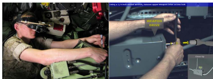
Fig. 28. Example of use of the system proposed by HENDERSON and FEINER [2009]: instructions are done with texts and virtual 3D models
