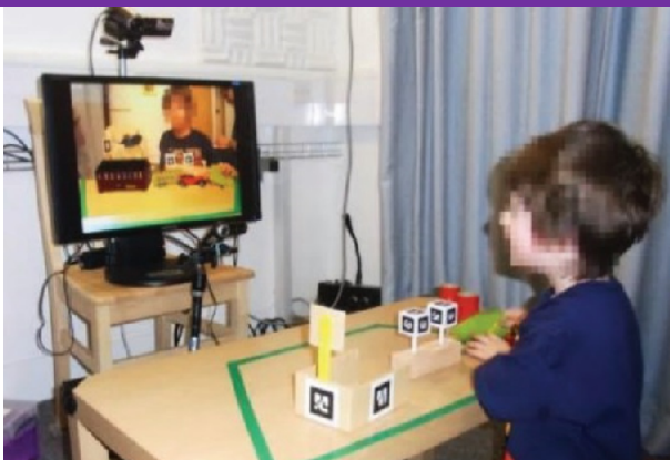
Figure 10: Augmented reality system associated with the use of real objects for autistic children. (Bai et al. , 2013).
