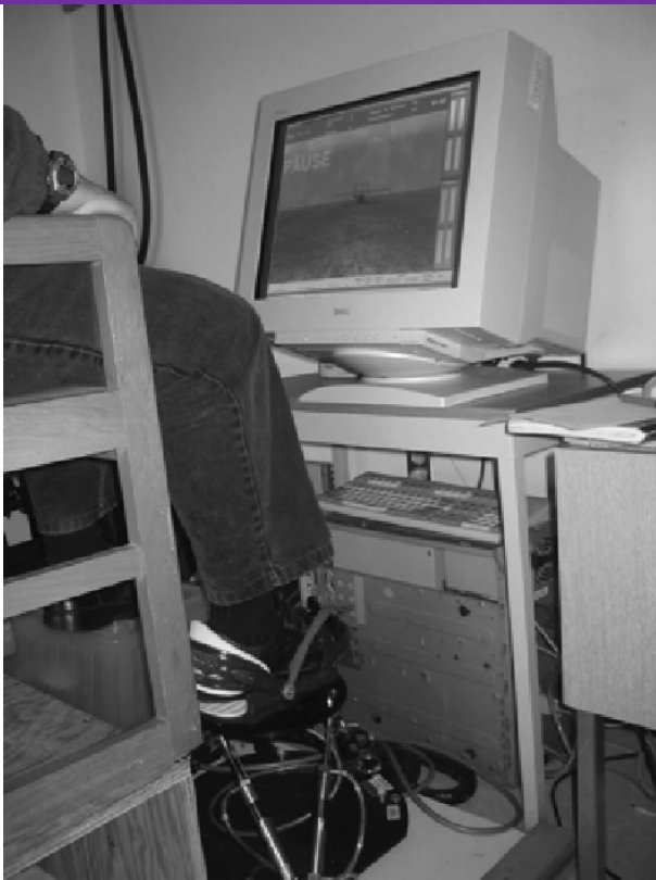
Figure 7: Rutgers Ankle robot for lower limbs interaction. (Mirelman et al. , 2009).
