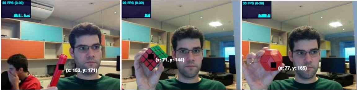
Figure 4-6: Library implementation of color tracking for different objects: On the left a red pencil marker; on the center a Rubik's magic cube [12] from the red face; and on the right a red Ball of Whacks [13].
